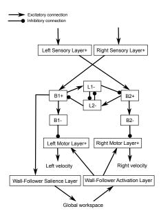
Fig. 3. Wall-following module
